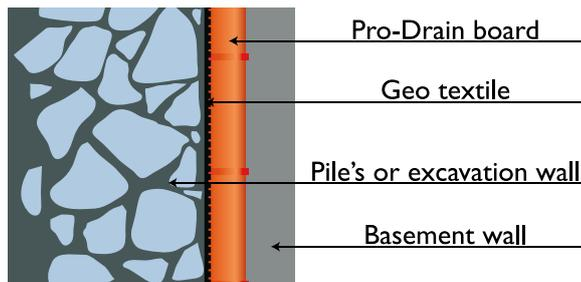
In some cases, when necessary, a geotextile can be used to prevent obstruction of the vertical channels by fine particles. In this situation, the geotextile is placed between the Pro-Drain and the excavation wall. (see picture of underground parking garage)
